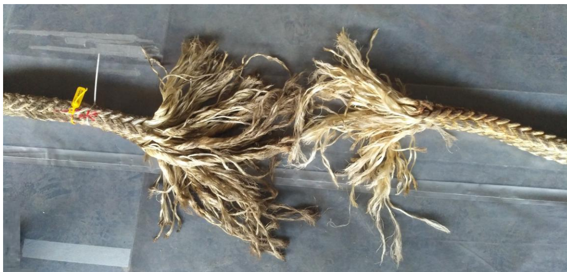
Figure no 1: Both parts of the mooring line after its breakage.
